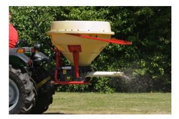
Vicon is introducing a new pendulum spreader. The PS225 pendulum spreader is replacing the PS203. The basic hopper capacity is increased up to 220 litres. The standard working width is 1-14 metres.
